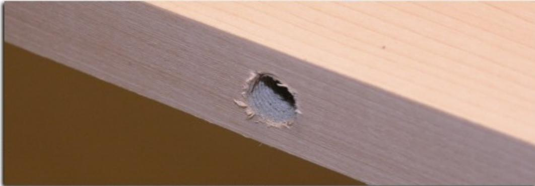
15. Use a brush or pipe cleaner to get the glue sealant down into the vacuum port hole. When it dries, apply a second coat so that the entire inside surface of the port has been sealed from the outside edge to the inside edge.
