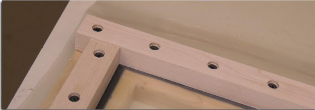
20. Select one of the remaining sides and attach the cleat. For the final side of the frame ask your helper again to hold the polyurethane film snug while you attach the last cleat.
