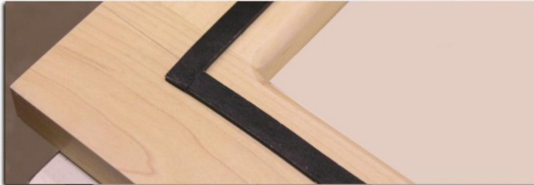
9. At this point, you'll need to make wooden "cleats" which will hold the polyurethane sheeting in place over the frame. Using  $\frac{3}{4}$ " thick lumber, cut 4 strips of wood that are 1" wide. They should be long enough to go around the frame using only 4 pieces. In the example above there would be two each of approximately 52" and 36".
