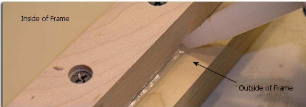
25. Apply a small amount of silicon to the threads on the brass tank fitting and attach it to the frame. It should be tight but be cautious that it is not so tight that it strips out the wood threads on the frame.
