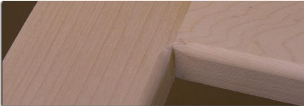
6. The maple lumber is mostly non-porous but under vacuum pressure, the microscopic pores that are present can allow leakage. To remedy this issue, mix 3 parts of yellow glue with 1 part water and apply this mixture with a paint brush to all sides of the frame (inside edge, outside edge, top, bottom, ends). When the glue "sealant" dries, lightly sand the frame with very fine sand paper and apply one additional coat of sealant.
